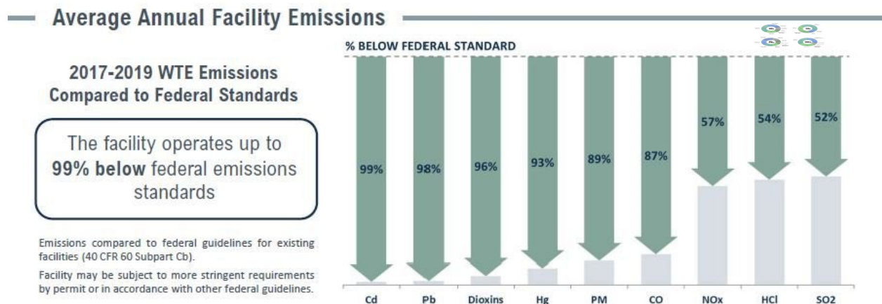
Figure 2-7: Covanta chart showing how high emissions limits are compared to actual emissions
